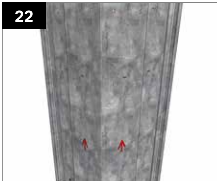
If cable management has been specified, the hup corner has an integrated insulated cable channel. The corner must be installed with the arrows pointing upwards.
