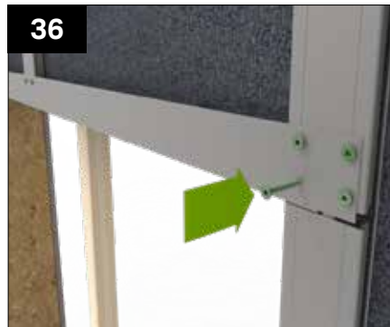
Ensuring the tray is level and propped at the centre (prop NOT SUPPLIED), fix the tray into the walling panel clips at both ends with four GPHS fixings and for each walling panels on the tray with two GPHS fixings through the pre punched holes.
